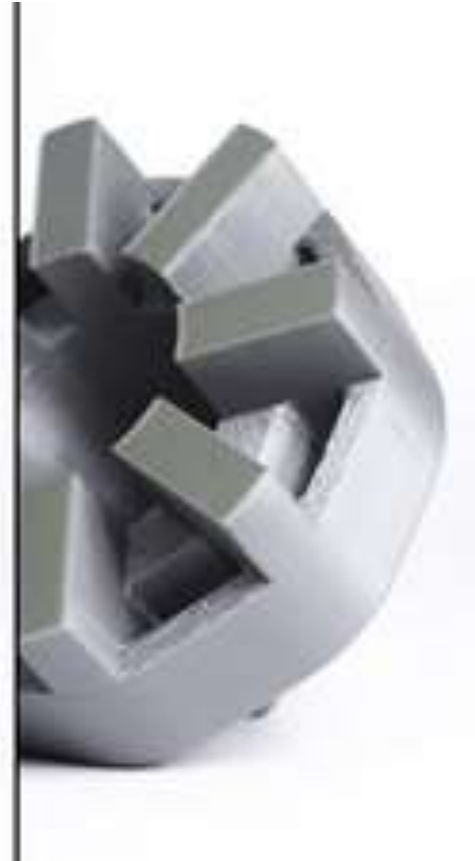
Support removed without much damage.
