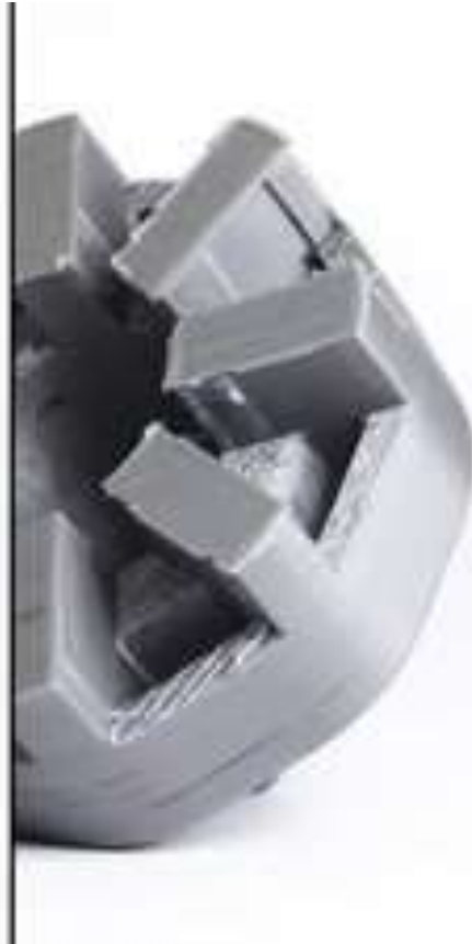
Support removal caused damage.
