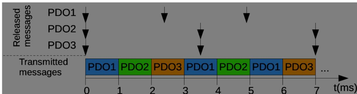
Here you can see that for first transmission of PDO3, it is released at  $t=0ms$ , and ends its transmission at  $t=3ms$ , resulting in a response time  $R=3-0=3ms$ . For the second transmission of
